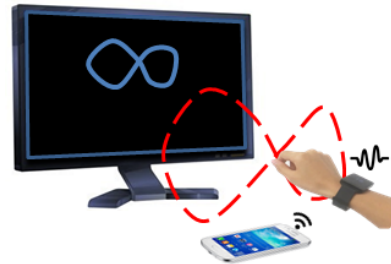
Fig. 1. Sound-driven wrist tracking with a smart watch-phone pair.
