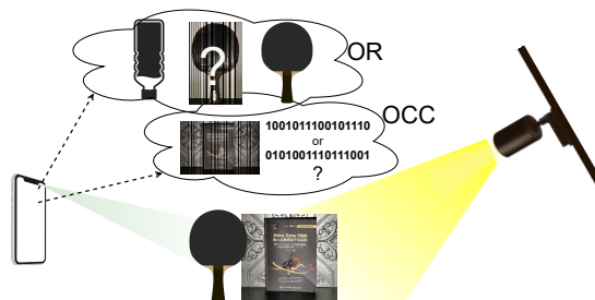
Figure 1: OCC demands an LED luminaire to emit information coded light. However, the mutual interference between the resulted light stripes and background objects affects both the object recognition (OR) accuracy and OCC decoding performance.
